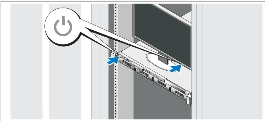
Press the power button on the system and on the optional monitor if used. The power indicators should light.
